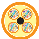
48-fibers (4 tubes of 12-fibers)
