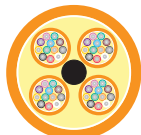
48-fibers (4 tubes of 12-fibers)
