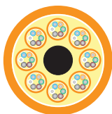
48-fibers (8 tubes of 6-fibers)
